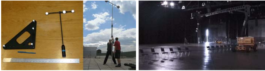
Fig. 4. Left: The standard sized calibration objects of length 15 inch. Right: Large 15 feet high wand.
